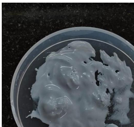
Fig2.4 Collected precipitate of ZnO MXene nanohybrid
