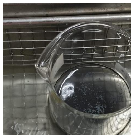
Fig2.5 Dispersion process of ZnO MXene nanohybrid
