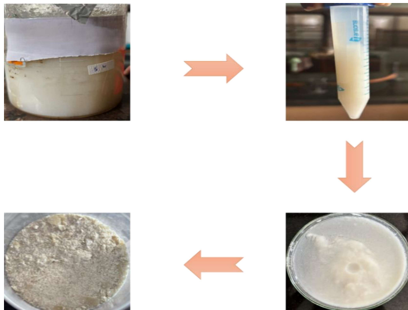
Fig.2.2 Preparation of MMT-CTAB Clay
