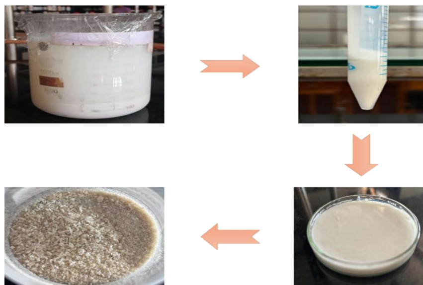
Fig.2.1 Preparation of Modified MMT-CTAB/Cinnamic acid Clay
