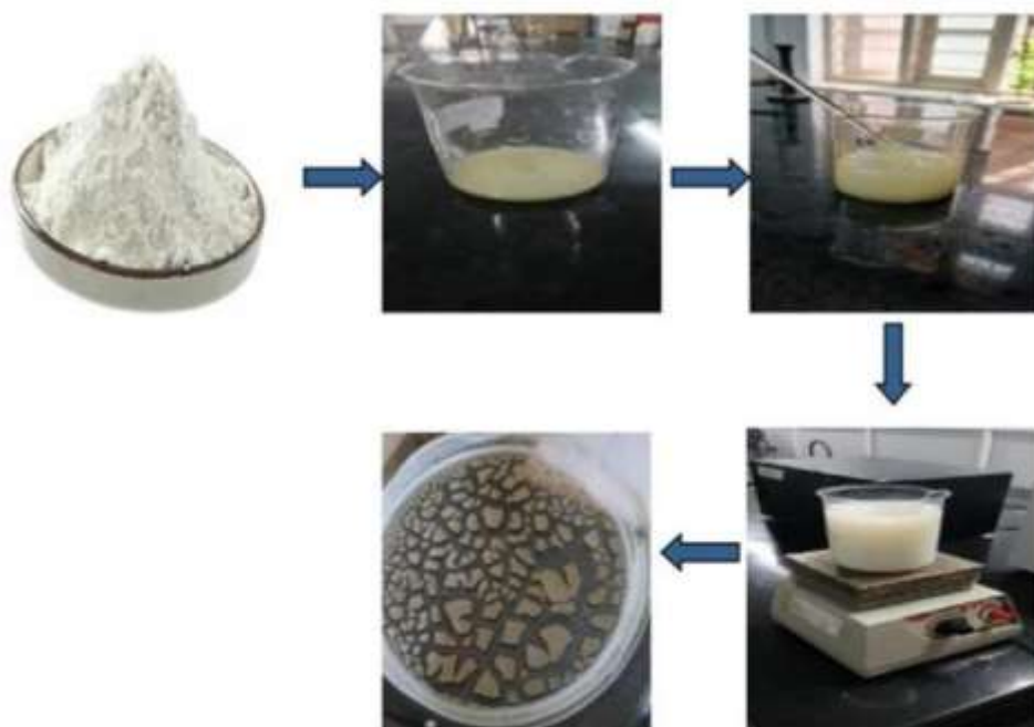
Fig 2.1: Modification of Montmorillonite clay
