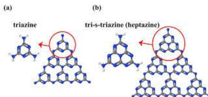
Fig.3a) Tri-s-triazine and 3b) triazine structures of g-C 3 N 4
