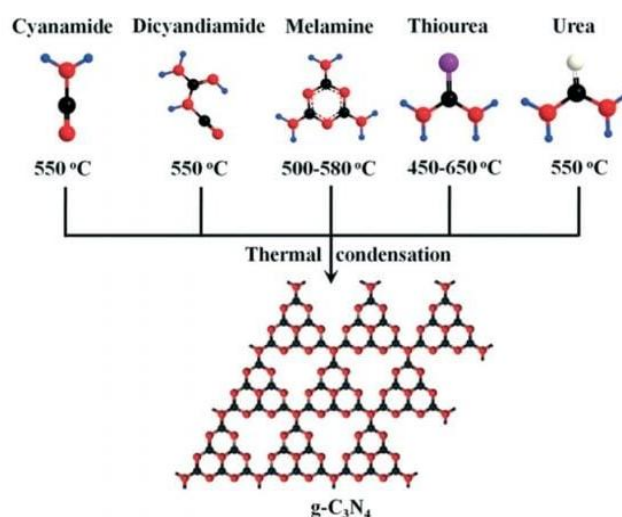
Fig.4 Schematic illustration of the main synthesis routes of bulk g\text{-C}_3\text{N}_4
