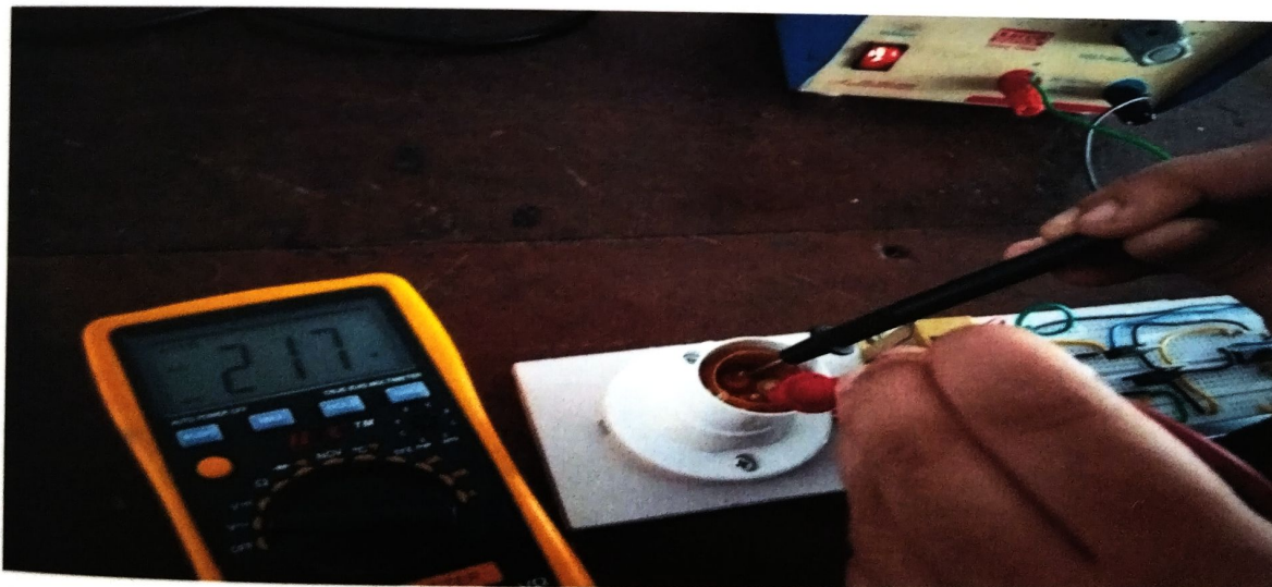
Fig 3.5 Output AC voltage 217 V
