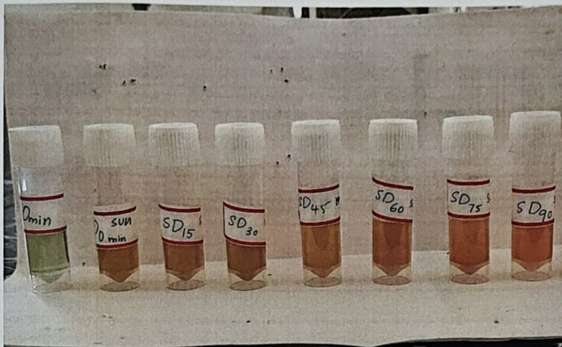
Figure:14 Visual changes in the Mixed dye solution (MB,MO & RhB) during Dark adsorption (0 to 90 minutes)
