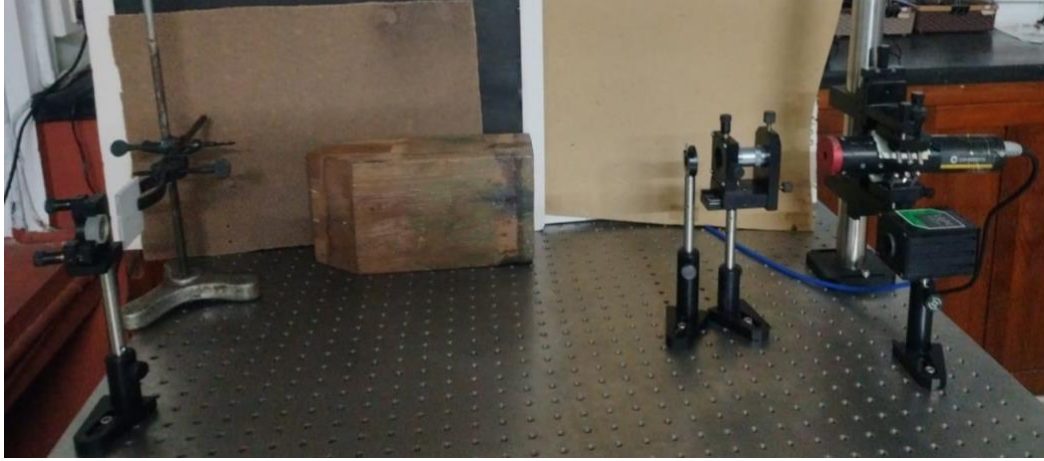
Fig(3.10) Entire experimental setup for non-destructive testing
