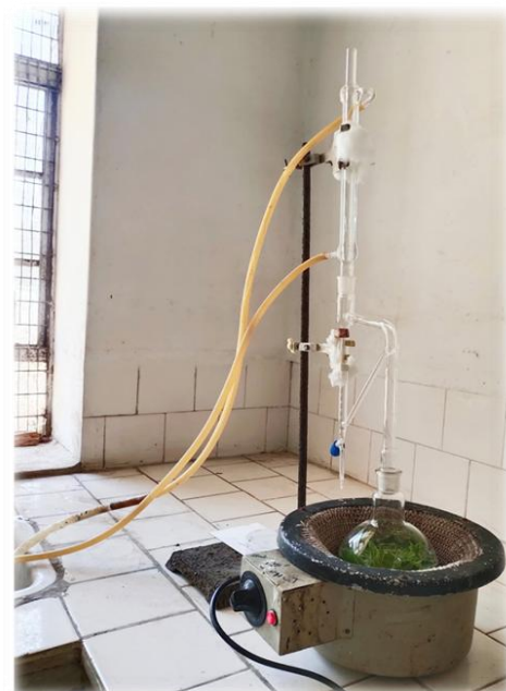
Plate 43. Experimental setup of Clevenger Apparatus
