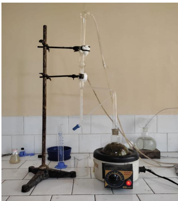
Figure 3. Essential oil extraction using cleavenger apparatus
