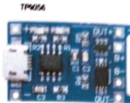
A lithium-ion battery charging module that regulates the charging process, providing overcharge protection and ensuring safe battery operation.
