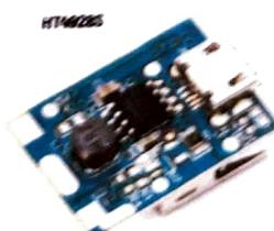
A boost converter module that steps up the battery voltage to a stable output, suitable for charging mobile devices via USB.
