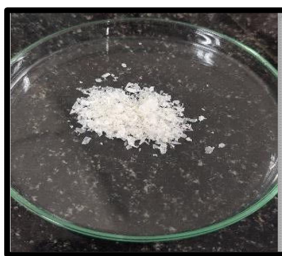
Fig. 3.1: Chitosan polymer taken in a Petri plate
