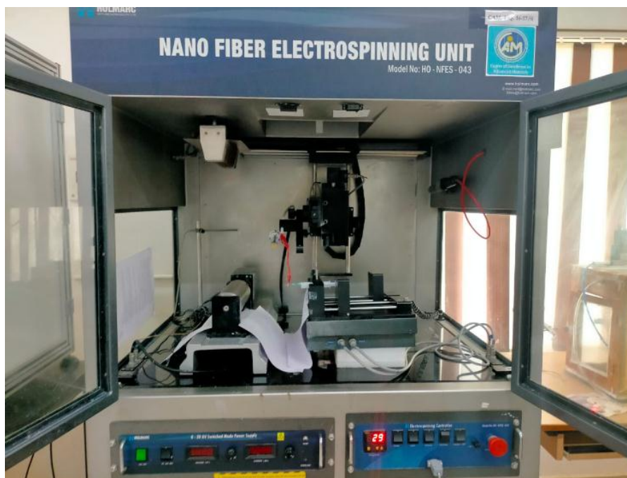
Fig 3.5. Electron Spinning Unit (Holmarc Opto-Mechatronics Ltd, India) used for the fabrication of membranes.
