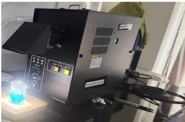
Fig 3.10. Photo degradation studies done using solar stimulator (SAN-EI Electric, Japan)
