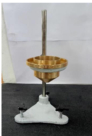
Figure 3.11: Cup Viscometer (used for measuring viscosity)
