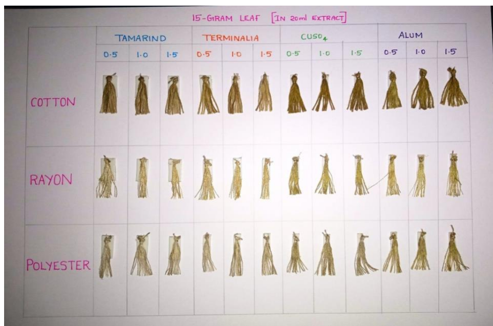
Fig. 10: Dyeing of cotton, rayon, and polyester fabric in dye concentration of 15 g by using various concentrations of mordants
