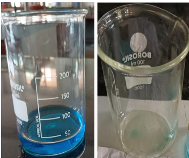
Fig 3.7 Methylene blue solution before adsorption and after adsorption BMOF
