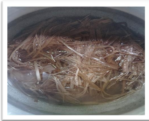
Plate.4a. Boiling of fibres
