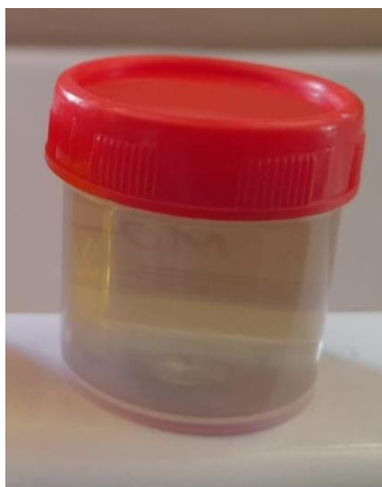
Fig 3.7 Methyl orange solution after adsorption by activated carbon for 10 min
