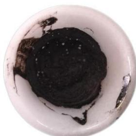
*Fig 2.2 Prepared Graphene oxide*
