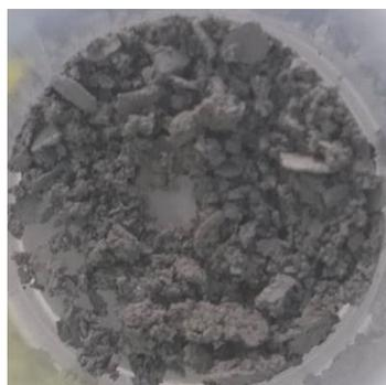
*Fig 2.3 Prepared ZnO-GO nanocomposite*
