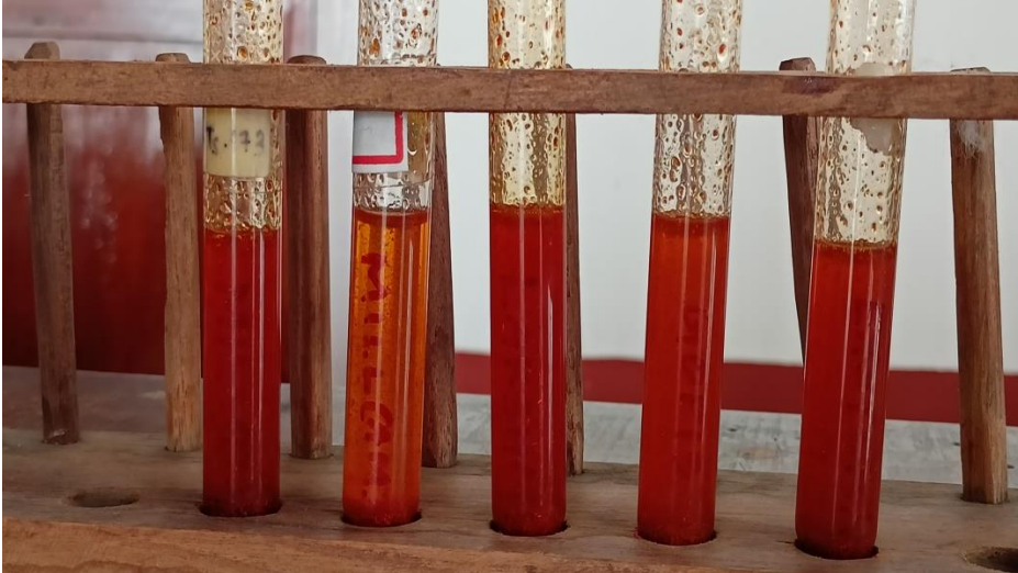
Fig 11-Test for Rhodamine B Detect the presence of Rhodamine B in chilli powder
