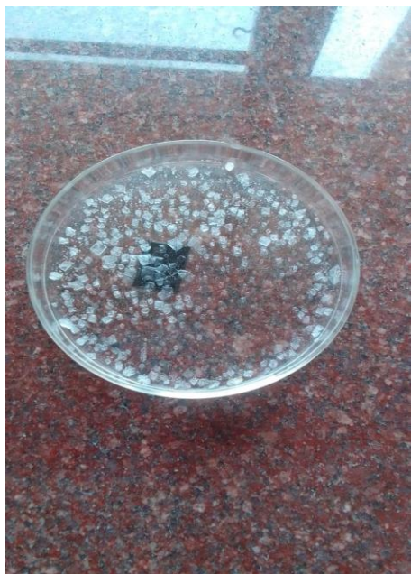
Image 2: TDS test – presence of the dissolved solvents in sample collected in petri plate
