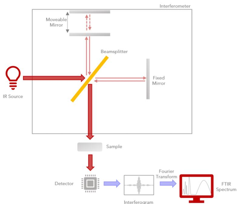
**Fig10. FTIR Instrumentation**[26].
