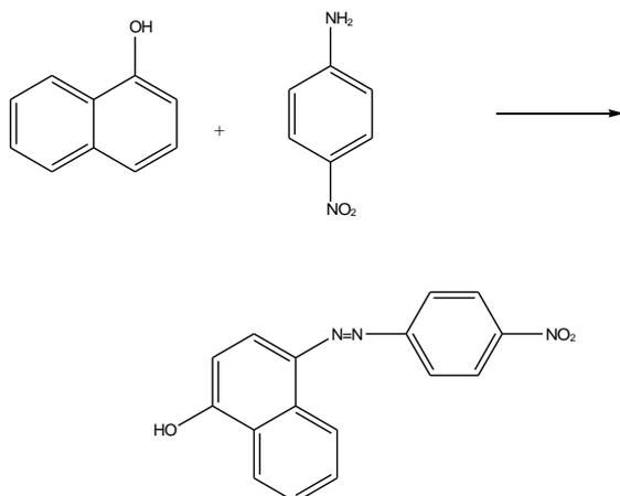
**Fig8. NAA synthesis reaction**
