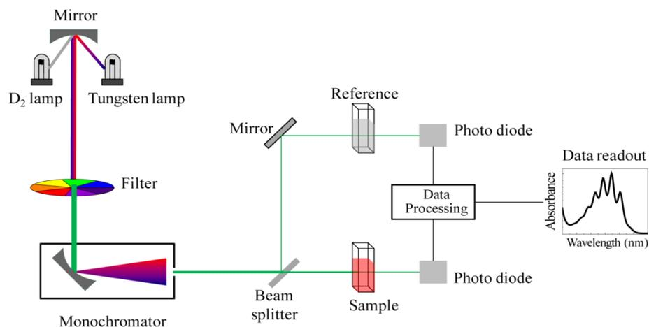
**Fig9. UV Instrumentation[25].**
