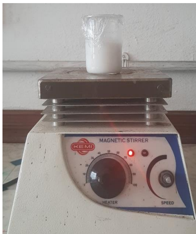
Fig. 2.3 Stirring of precipitate dissolved in deionized water for 3 hours in a magnetic stirrer
