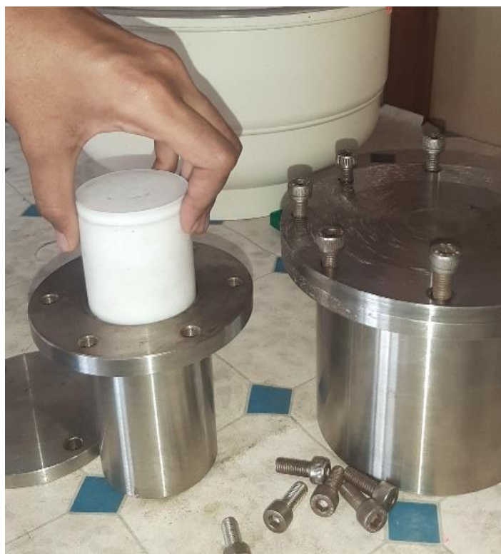
Fig. 2.2 Placing the white precipitate in teflon-lined flask for heating it for 6 hours at 160°C
