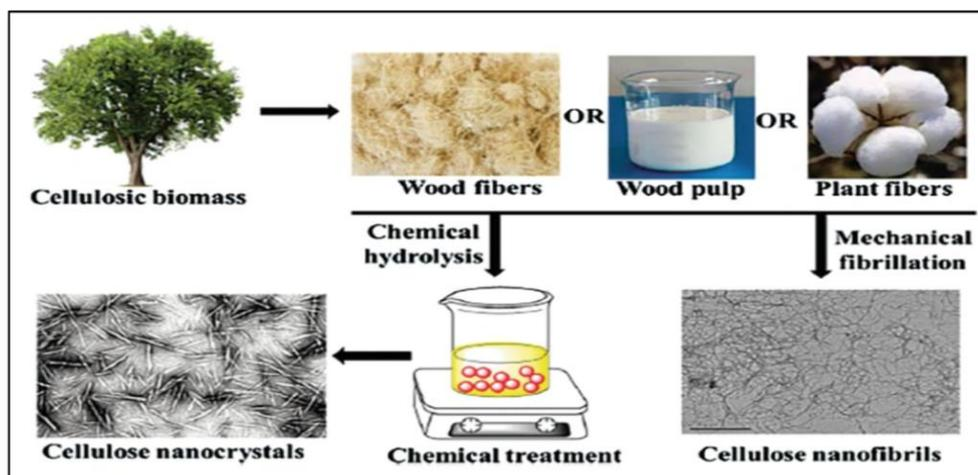
Fig.3 Synthesis of Cellulose Nanocrystals
