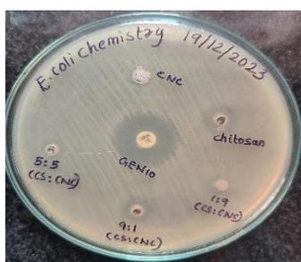
Fig.21 Antibacterial activity of CNC, Chitosan [CS], 1:9 [CS:CNC], 9:1 [CS:CNC], 5:5 [CS:CNC] against *E. coli*
