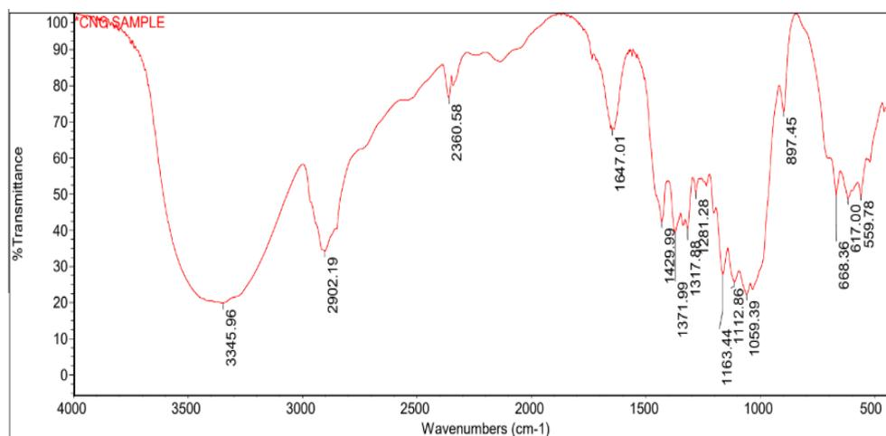
Fig.20 FTIR spectra of Cellulose nanocrystals
