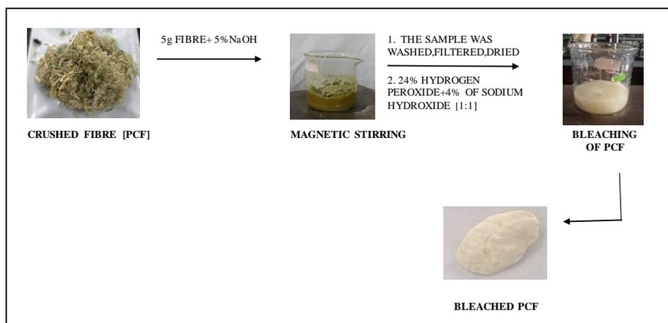
Fig10 FLOW CHART SHOWING THE ALKALI PRE-TREATMENT PROCEDURE
