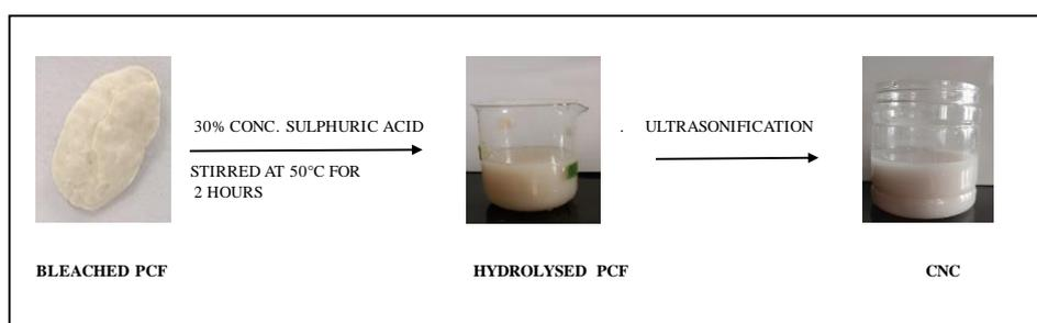
Fig.11 FLOW CHART SHOWING THE ACID HYDROLYSIS PROCEDURE
