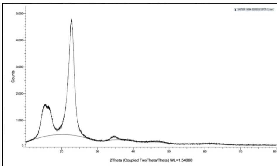
Fig.16 XRD Graph of Cellulose Nanocrystals
