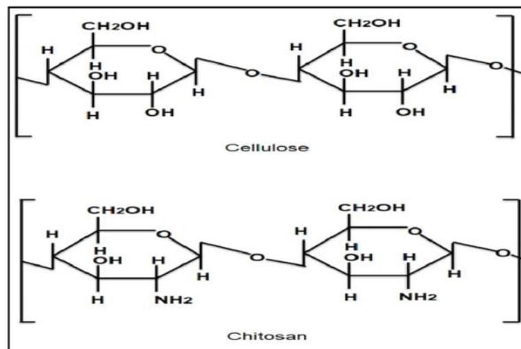
Fig.8 Structure of Cellulose and Chitosan
