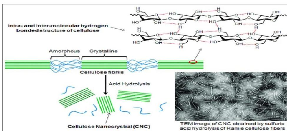
Fig.2 Graphical depiction of a CNC (cellulose nanocrystal) derived from cellulose chain.
