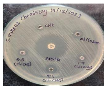
Fig.22 Antibacterial activity of CNC, Chitosan [CS], 1:9 [CS:CNC], 9:1 [CS:CNC], 5:5 [CS:CNC] against *S. aureus*
