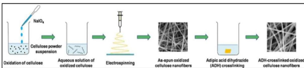
Fig.6 Synthesis of Electro-spun cellulose Nanofibers
