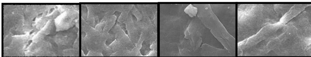
Fig.17 SEM images of Cellulose Nanocrystals
