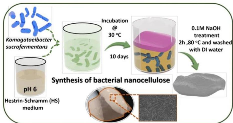
Fig.5 Synthesis of Bacterial Nanocellulose
