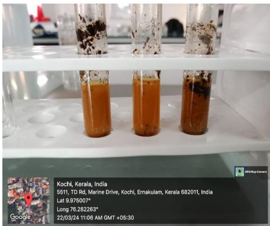
Fig 4.6: Formation of turbidity in Dragendorff's test for alkaloids
