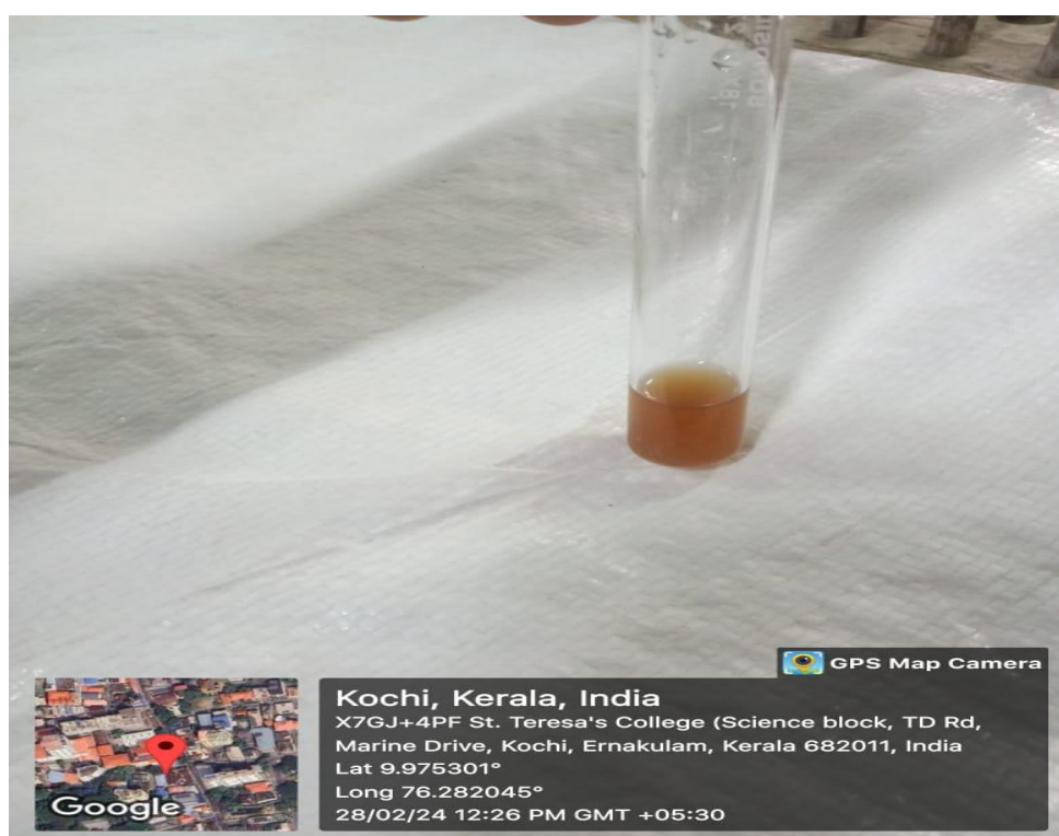
Fig 4.14: Deep yellow colour in Alkaline reagent test for tannins
