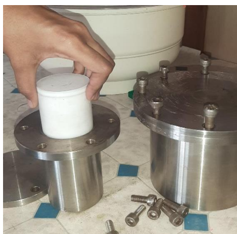
Fig. 2.2 Placing the white precipitate in teflon-lined flask for heating it for 6 hours at 160°C
