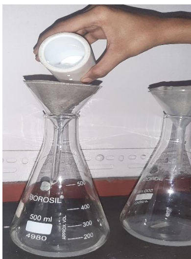
Fig. 2.3 Filtration and washing with deionized water
