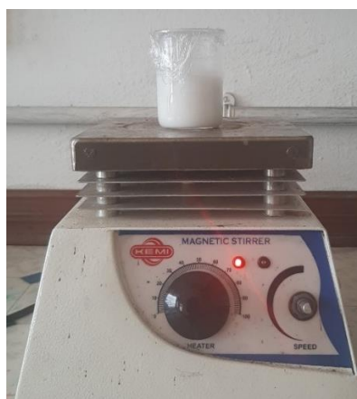
Fig. 2.3 Stirring of precipitate dissolved in deionized water for 3 hours in a magnetic stirrer
