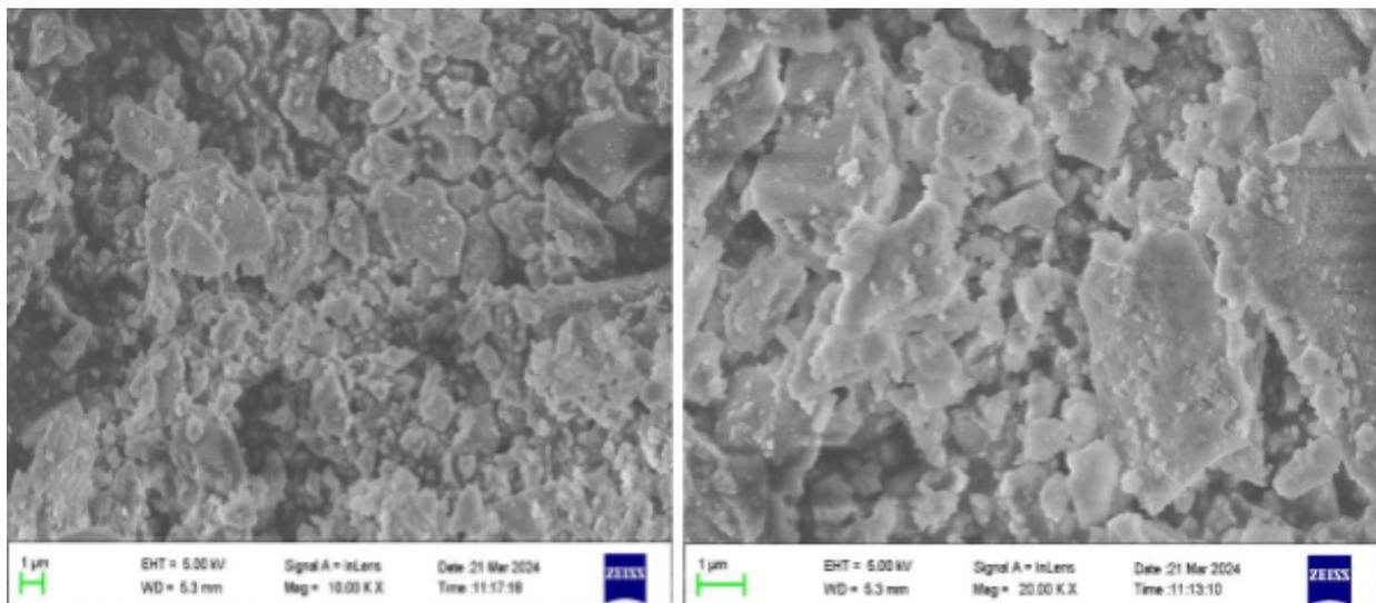
Figure SEQ Figure \\* ARABIC 16 SEM image obtained for the synthesized amorphous silica nanoparticles
