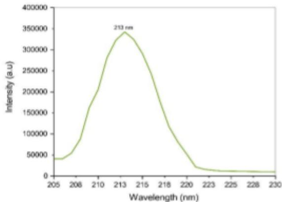
Figure SEQ Figure \\* ARABIC 18 Excitation spectrum with a peak at 213 nm
