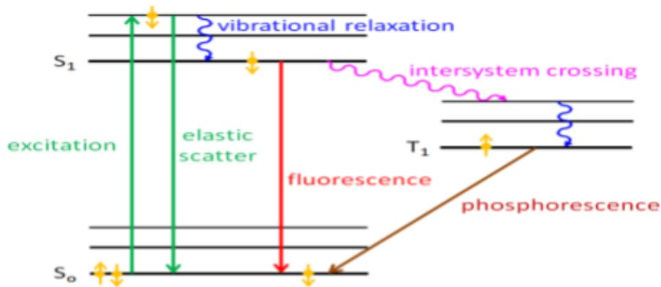
Figure SEQ Figure \\* ARABIC 9 Schematic representation of photoluminescence
