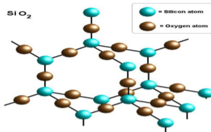
Figure SEQ Figure \\* ARABIC 1 Structure of silica
