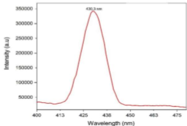
Figure SEQ Figure \\* ARABIC 18 Emission spectrum with a peak at 430 nm when excited at a 213 nm wavelength
