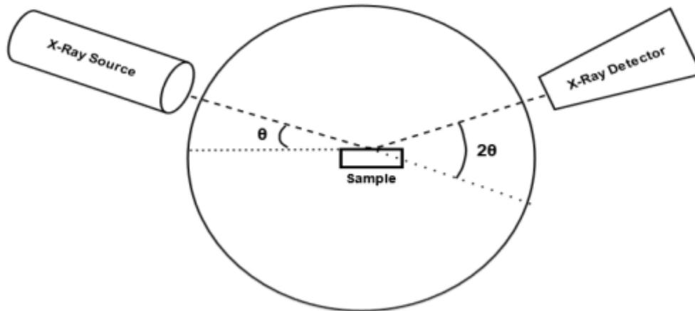
Figure SEQ Figure \\* ARABIC 4 XRD instrumentation
