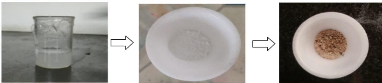
Figure SEQ Figure \\* ARABIC 12 (a) gelation (b) after heating at 100 degree celcius for 2 hours (c) after calcination at 500 degree celcius for 4 hours
