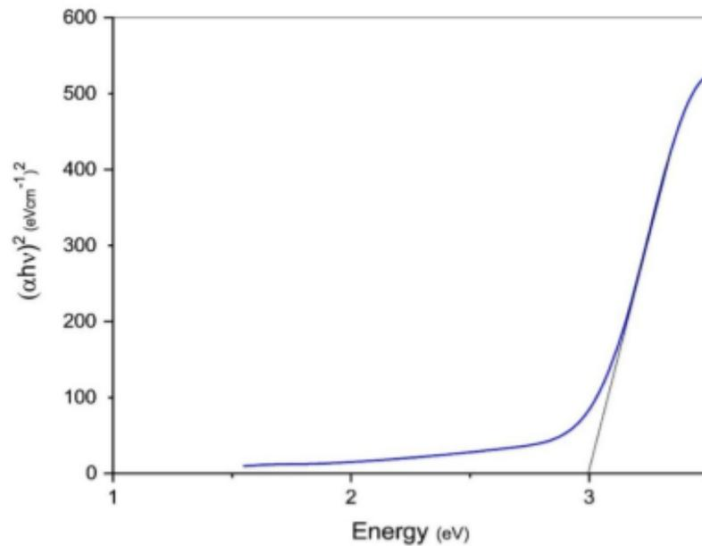
Figure SEQ Figure \\* ARABIC 15 Tauc plot of the synthesized nanoparticles showing a 3eV bangap energy
