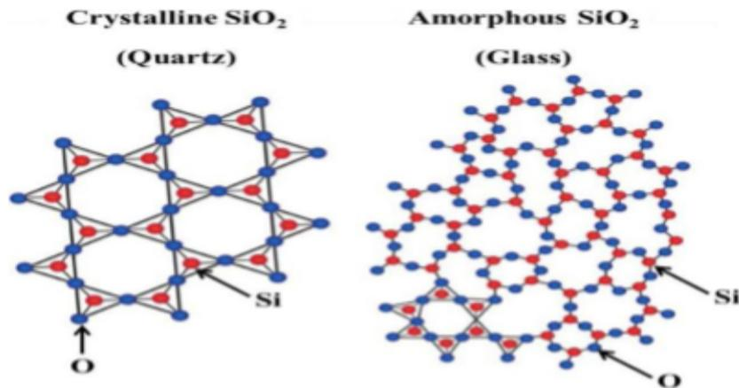
Figure SEQ Figure \\* ARABIC 2 Crystalline and amorphous structure of silica
