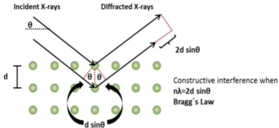
Figure SEQ Figure \\* ARABIC 3 X-Rays diffracted by atoms within a crystal
