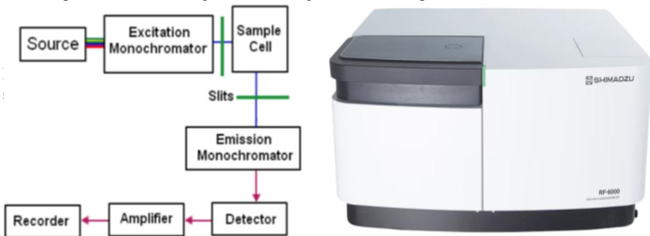
Figure SEQ Figure \\* ARABIC 10 Block diagram and a real picture of spectrofluorometer
