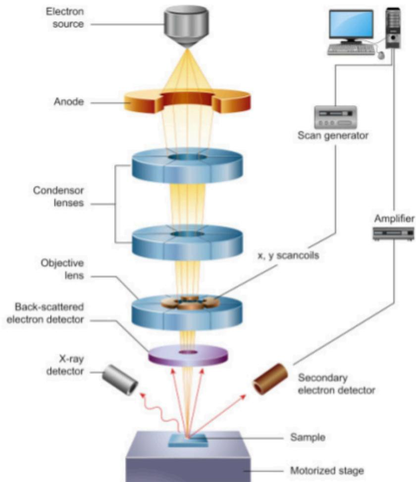
Figure SEQ Figure \\* ARABIC 6 SEM instrumentation
