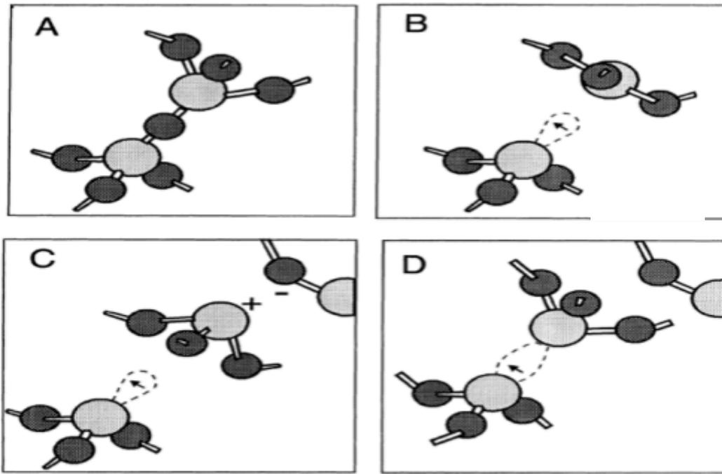
Figure SEQ Figure \\* ARABIC 22 (A)Fragment of a perfect lattice (B)Asymmetrically relaxed oxygen vacancy with a localized unpaired electron in a sp<sup>3</sup>-like orbital of a silicon atom (C)and(D)Two different types of bonding that the two separated silicon atoms can form
