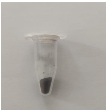
Fig 2.3 Obtained Cu/Cu 2 O/CuO nanocomposite.
