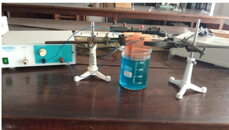
Fig 2.1 electroplates immersed in copper sulfate solution and connected to power supply.
