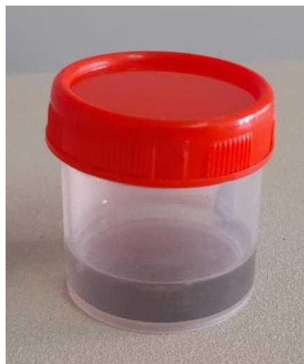
Fig 3.6 Methyl orange solution after adsorption by activated carbon for 20 min
