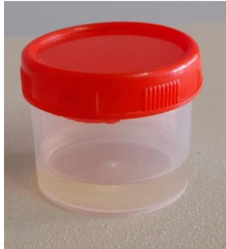
Fig 3.5 Methyl orange solution after adsorption by activated carbon for 30 min.
