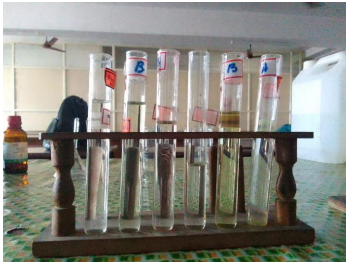
Image 4: Nitrate estimation of samples collected from marine drive
