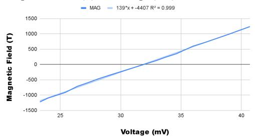
slope=139  $\times 10^3 \times 10^{-4} \, \text{T/V}$ =13.9 T/V thickness,t=5 $\times 10^{-4}$  m  $R_H$ = ( $V_H$ t/ $I_c$ B) = t/ $I_C$  $\times$ slope = (5 $\times 10^{-4}$ )/((2 $\times 10^{-3}$ ) $\times 13.9$ ) = 0.0179856 m $^3$ C $^{-1}$   $R_H$  is positive. This means, the given material is p type semiconductor.
