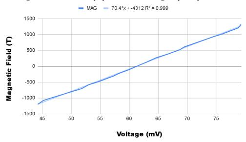
$$\begin{split} Slope &= 70.4 \ \hbox{$\times$} 10^3 \ \hbox{$\times$} 10^{\text{-4}} \ T/V = 7.04 \ T/V \\ Thickness, t &= 5 \hbox{$\times$} 10^{\text{-4}} \ m \\ R_H &= (V_H t/I_c B) = t/I_c \hbox{$\times$} slope = (5 \hbox{$\times$} 10^{\text{-4}})/((4 \hbox{$\times$} 10^{\text{-3}}) \hbox{$\times$} 7.04) = 0.01775568 \ m^3 C^{\text{-1}} \end{split}$$
