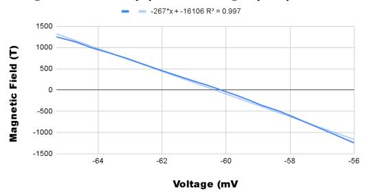
$slope= -267 \times 10^3 \times 10^{-4} \, T/V = -26.7 \, T/V$  thickness,t=6.4×10<sup>-4</sup> m  $R_H = (V_H t/I_c B) = t/I_c \times slope = (6.4 \times 10^{-4})/((2 \times 10^{-3}) \times -26.7) = -0.11985 m^3 C^{-1}$  Here  $R_H$  is negative, which means the given material is n type semiconductor.
