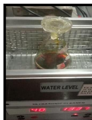
SONICATED FOR 40 MINS AT 25-40°C
