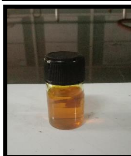
OBTAINED NANOCURCUMIN SOLUTION IN ACETONE
