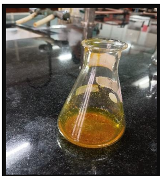
0.5g TURMERIC POWDER DISSOLVED IN 10 ml ACETONE
