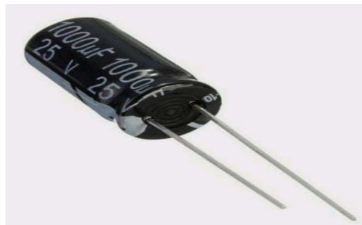
Fig 11. Electrolytic capacitor (1000 µF)
