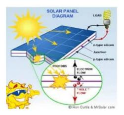
The solar cell works on the principle of the photovoltaic effect. Sunlight is composed of photons, or "packets" of energy. These photons contain various amounts of energy corresponding to the different wavelengths of light. When a photon is absorbed, the energy of the photon is transferred to an electron in an atom of the cell.
