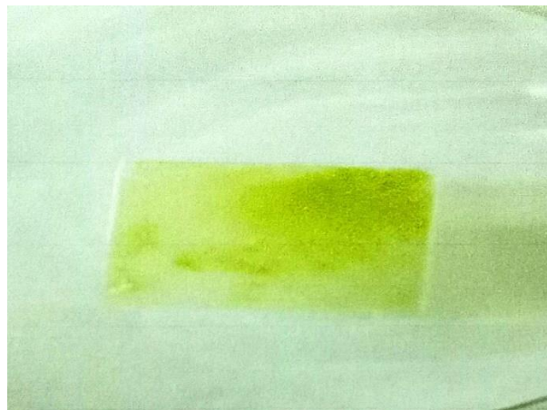
Figure.13. Development of biofilm on the surface of ITO at 3 rd day of inoculation
