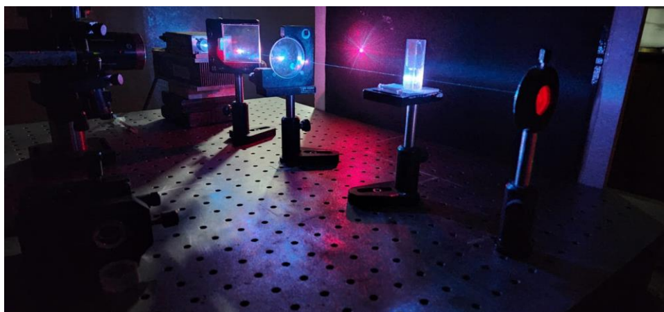
Figure 4. 2 The experimental set up of dual beam thermal lens technique
