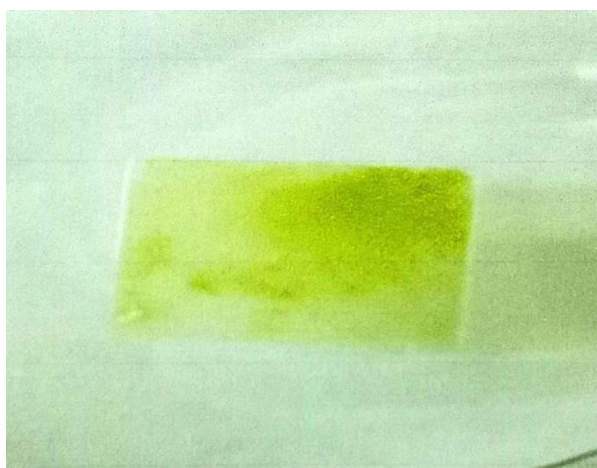
Figure 13: Development of biofilm on the surface of ITO on the 3 rd day of inoculation.
