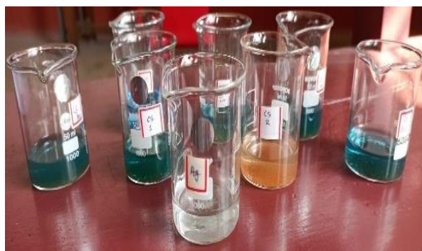
Image 3.17 Photo degradation of methylene blue dye by ZF/Ag nano composite (Sample CS2)
