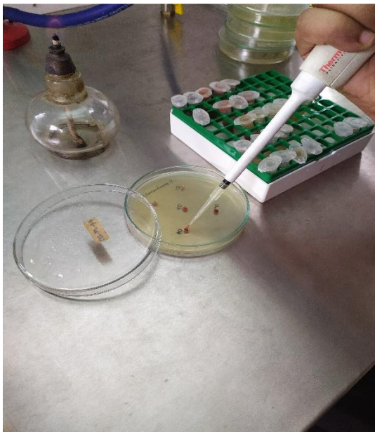
Fig.B. Wells were labelled and 20 \mu L of nanoparticles were loaded into corresponding wells.
