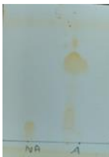
Fig. 23. TLC of acetylated and non acetylated samples (Solvent system: Hexane: Ethylacetate 8:2)
