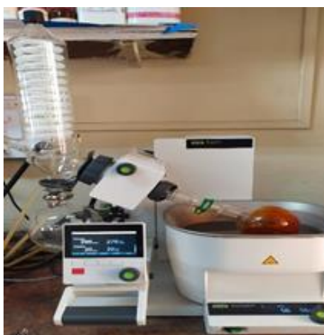
Fig. 15. Concentrating hexane soluble extract in rotary evaporator
