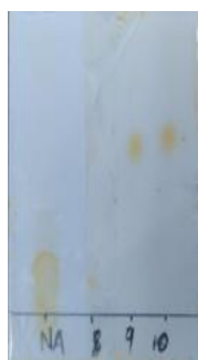
Fig. 24. TLC of fractions separated by column chromatography
