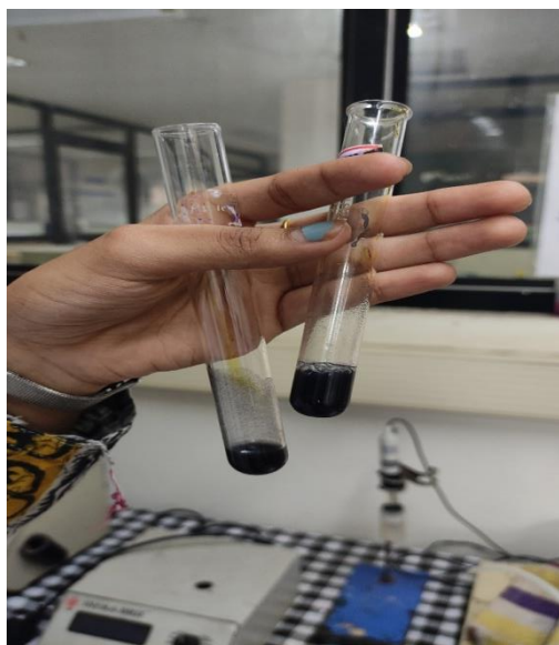
Fig .9 precipitate turned blue black indicating presence of starch
