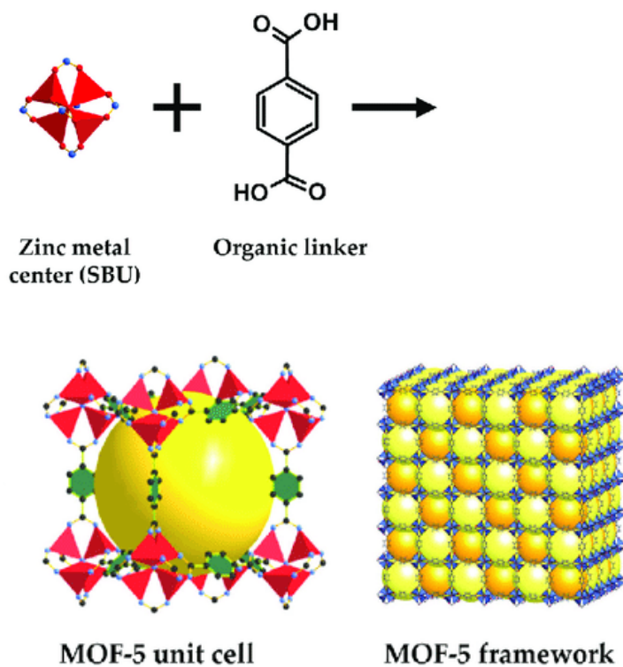
Figure1.3: Structure of Zn MOF(MOF-5)
