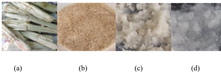
Fig3.1. Physical appearance of collected sugarcane bagasse (a), crushed sugarcane bagasse (b), extracted cellulose (c) and nanocrystals (d)
