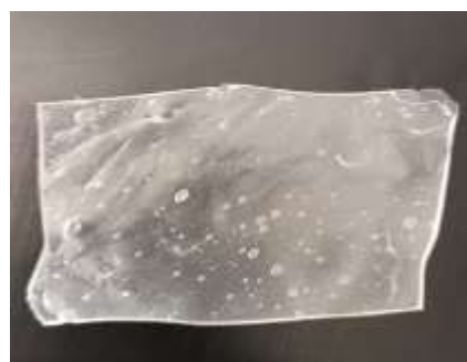
Fig 10 (d): CSGS (corn starch + acetic acid + 2.5ml glycerol + 2.5 g sorbitol)
