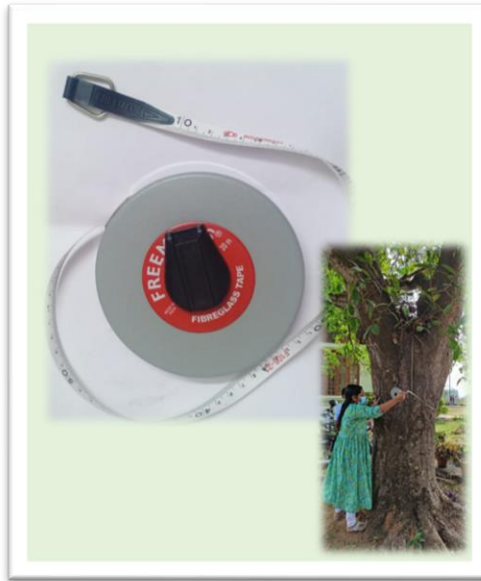
Measurement of Diameter using Tape
