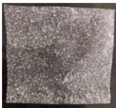
*Fig 11 (c):CS<sub>1</sub> b (Corn starch + sorbitol+ acetic acid + 2g CESP)*
