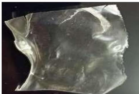
*Fig 4: bio-plastic obtained from corn starch + acetic acid*
