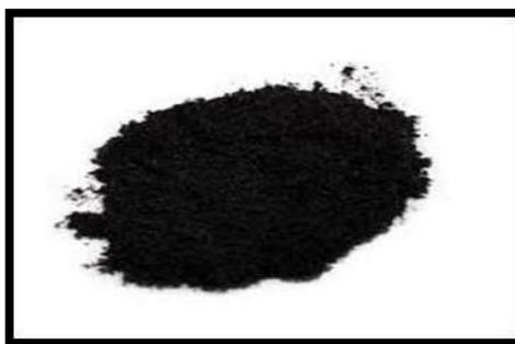
*Fig 6: Graphene oxide prepared by Hummer's method*
