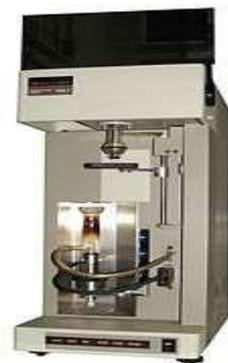
*Fig 7: Thermo gravimetric analyser*
