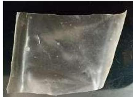
*Fig 10 (b): CS<sub>1</sub> (corn starch + acetic acid + 5 g sorbitol)*
