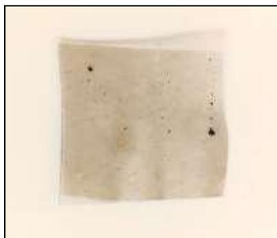
*Fig 11 (a): CS<sub>1</sub>(GO<sub>1</sub>) {corn starch + acetic acid+ 5 g sorbitol + 0.1 g GO}*
