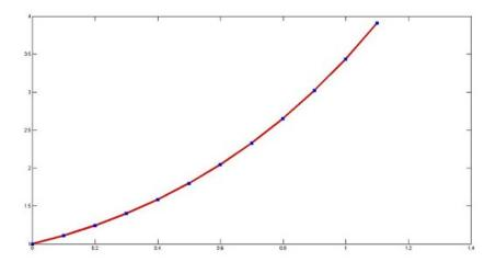
The red line represents the original solution and the blue dots represent the solution got by R K method. One of the merit of this method is that the operation is identical whether the differential equation is linear or nonlinear. R-K method has been constructed so as to give better accuracy and it requires only the function values at some selected points on the sub interval. Thus we can conclude that R-K method have better performance over other methods.
