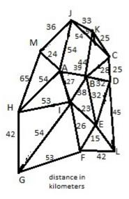
Let us assume that a radio station has a broadcast range of fifty kilometers. What is the least number of stations in a set which dominates within distance 50 all other vertices in this graph? A set B,F,H,J of cardinality four is indicated in the following figure 2.
